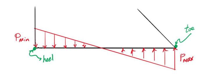
No tension should be permitted at any point of the dam. The eccentricity **e** should be less than  $\frac{B}{6}$ . ( $e < \frac{B}{6}$ ). Thus, the result should always lie within the middle third of the base.
