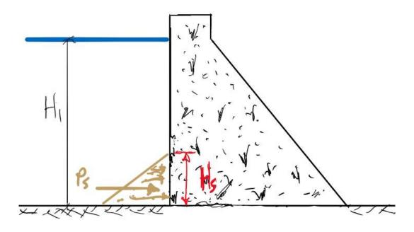
Ø: is the angle of internal friction of Soil, and cohesion is neglected.
